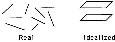
Fig. 15. Arrangements in space of platelet fillers.
